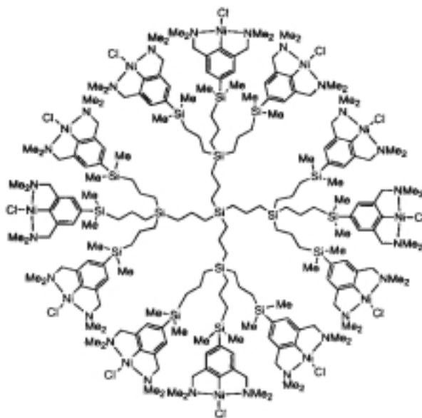
Figure 3.2. Dendrimers having NCN pincer systems directly attached to the peripheral silyl groups.
